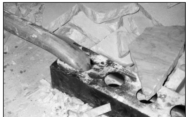
Picture 6.7 – Example of buckled tube due to overloading.
